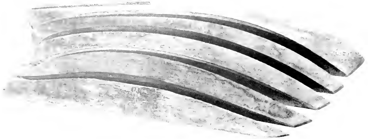
STANDARD LIFT HALF-MODEL WITH FASTENERS REMOVED AND THE LIFTS SLIGHTLY SPREAD. A quarter deck rail lift is shown. This model, in the author's collection, is of a Connecticut schooner, name unknown, of the pilot-boat type, built at Westbrook, Connecticut, about 1825-30. ( Smithsonian photo 45608-t. )
